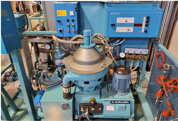
Fig. 5 Transfer condition with the MMPX oil separator in the machinery laboratory
