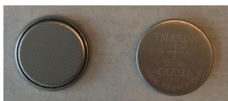
Figure 13. An assembled coin cell
