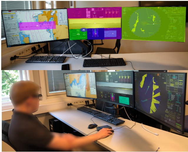
Figure 17. Experimental setup: Radar, Bridge (main interface), ECDIS
