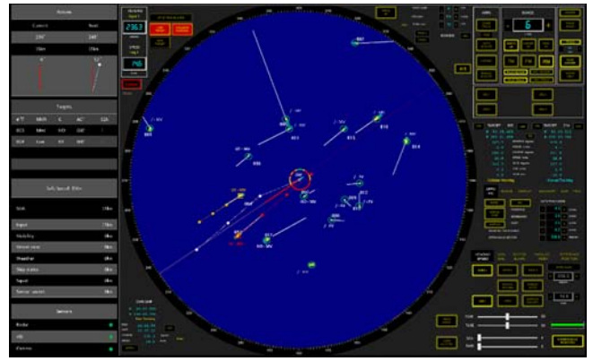
Figure 9. Traffic situation with transparency information overlaid (decision selection + information analysis + information acquisition).
