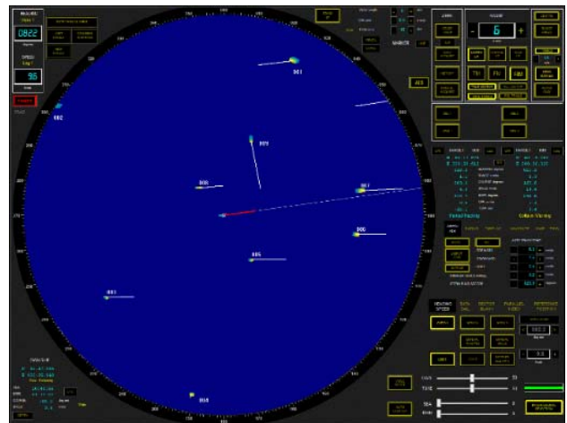
Figure 4. Own ship is in a crossing situation in open waters where it is required to stand-on. The situation is of high complexity as there are restrictions to the target ship's avoidance manoeuvrability (the ship crossing at port side).
