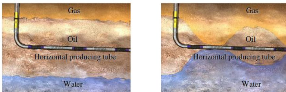
Figure.1.1 – Multiphase flow in transportation pipes due to water and gas coning: (a) Initial condition, (b) After production (Kumara 2010).
