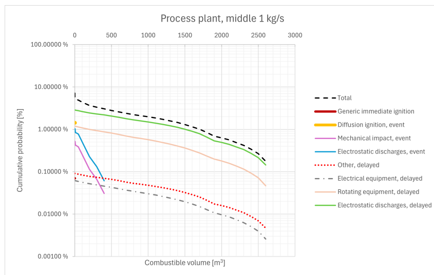
Figure 8.18: Contributors to the total ignition probability where the ignition probability is plotted against the cloud volume, for the middle leak with 1 kg/s leak rate for the process plant geometry.
