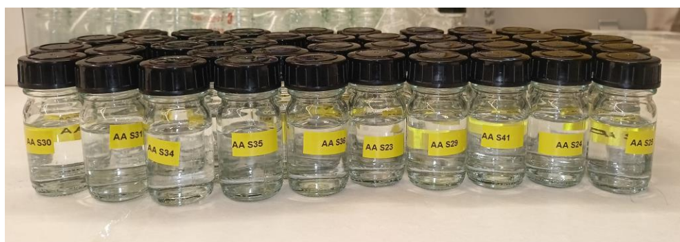
Figure 4.3: All 41 Unloaded prepared Sample (AMP+PZ+Water).
