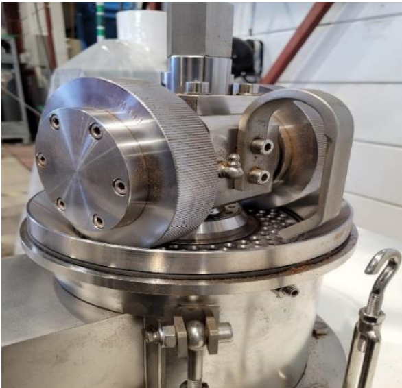
Figure 3.6 Die and Roller Arrangement
