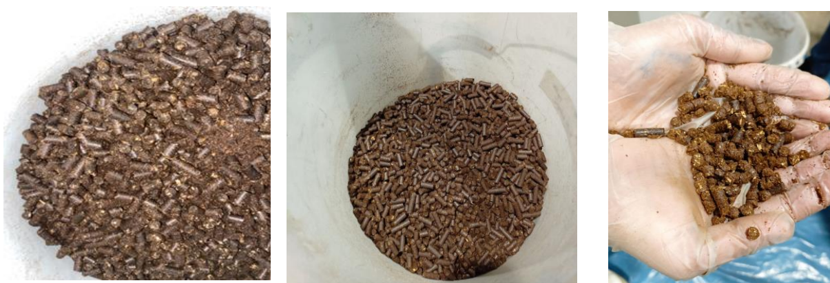
Figure 4.2 Pellets with moisture content of 9%,10% and 13% (from left)
