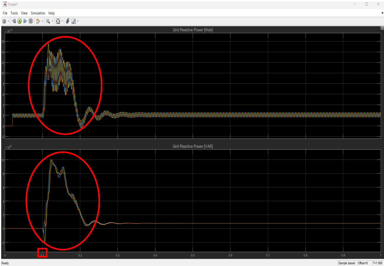
Figure 5.9: Simulink results of grid active and reactive power before peak shaving.
