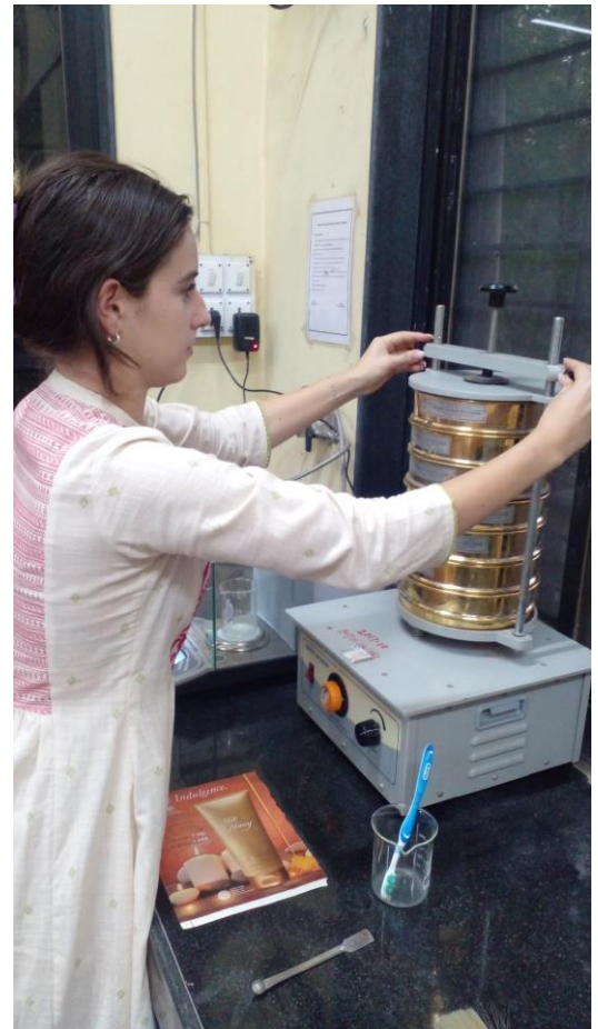
Figure 12. During the sieve analysis, we employed mesh sizes from 4 to 240 on the ASTM U.S. Standard scale representing 4760 to 53µm, and a sieve shaker to speed up the process.
