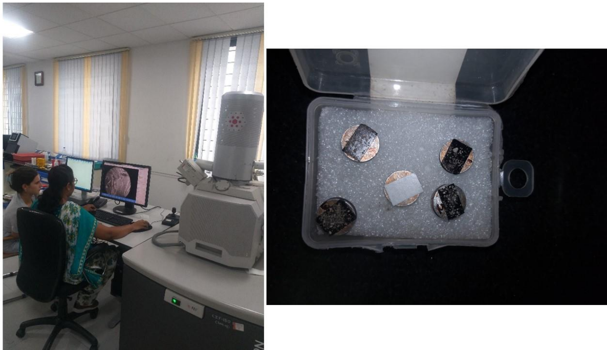
Figure 13. SEM equipment on the left side. On the right side, the Studs with the grains spread ready to be introduced into the SEM machinery.
