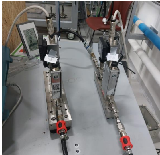
Figure 3.5: Gas handling unit. The left one controls the hydrogen flow and the right one controls air flow.
