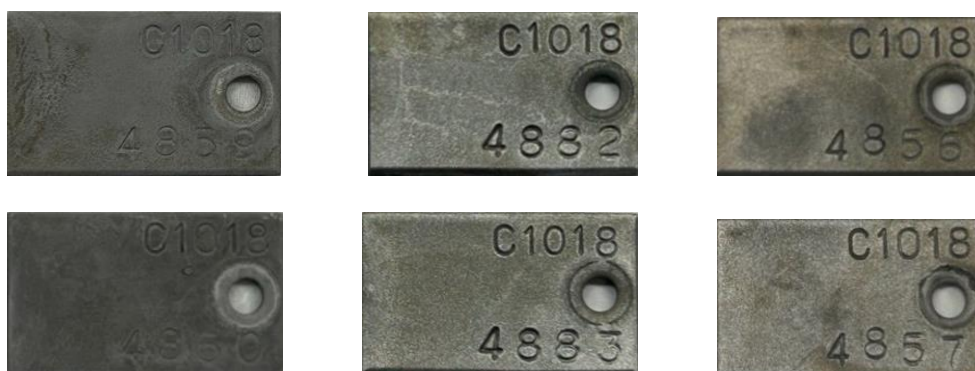
Figure 4.18 Coupons after 72 hours immersion in the presence of CO 2 /H 2 S.
