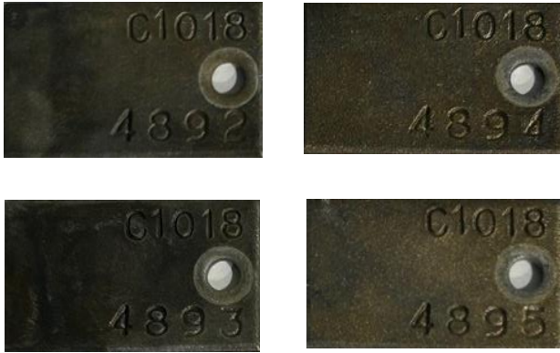
Figure 4.24 Coupons after 72 hours immersion in the presence of 99.965% CO 2 / 0.035% H 2 S.
