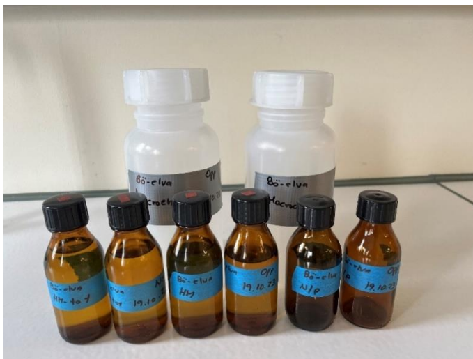
Figure 2.3.1 Sampling containers for sampling. 1000 mL PE bottle for macro-chemistry (in the back row). 100 mLr brown glass bottles for Tot-N and Tot-P (acidified by H_2SO_4 ) and heavy metals (acidified by HNO_3 ).
