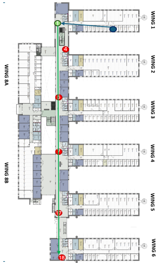
Figure 10.4 Layout drawing of second floor, where arrows indicate the LOS from relay to node
