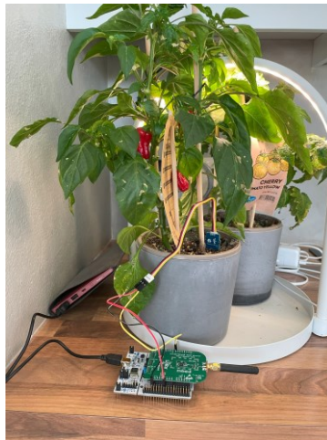
Figure 12.5 Test scenario: The moisture sensor placed in a pot with soil and a red pepper plant, with the Nucleo board powered by a power bank
