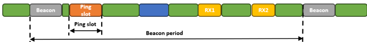
Figure 2.5 Illustration of Class B device operation, reproduced from [24]
