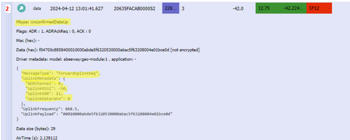
Figure 6.3 Content of join request uplink message, forwarded by the relay
