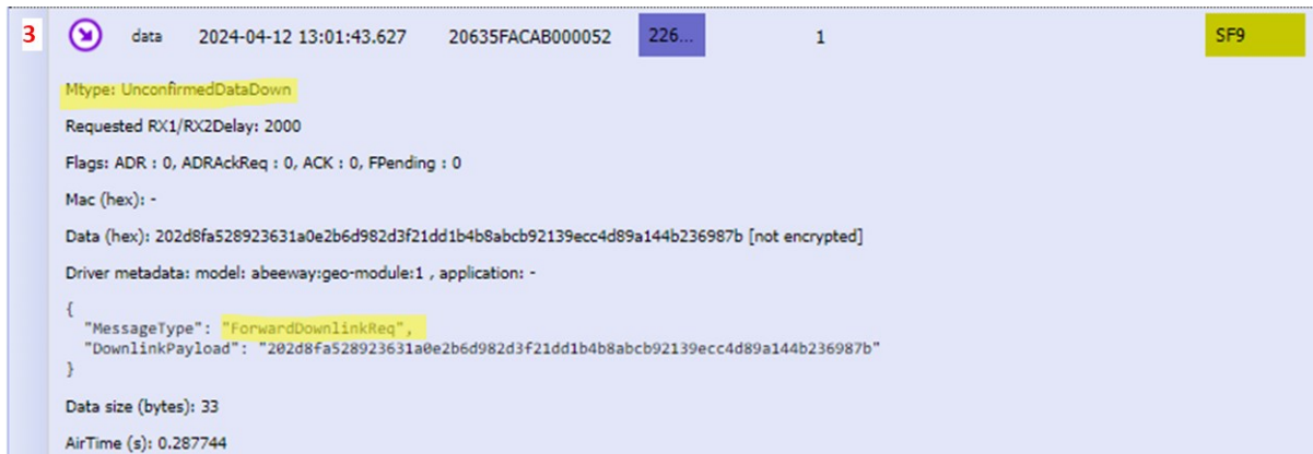
Figure 6.4 Content of LNS downlink reply message to the relay
