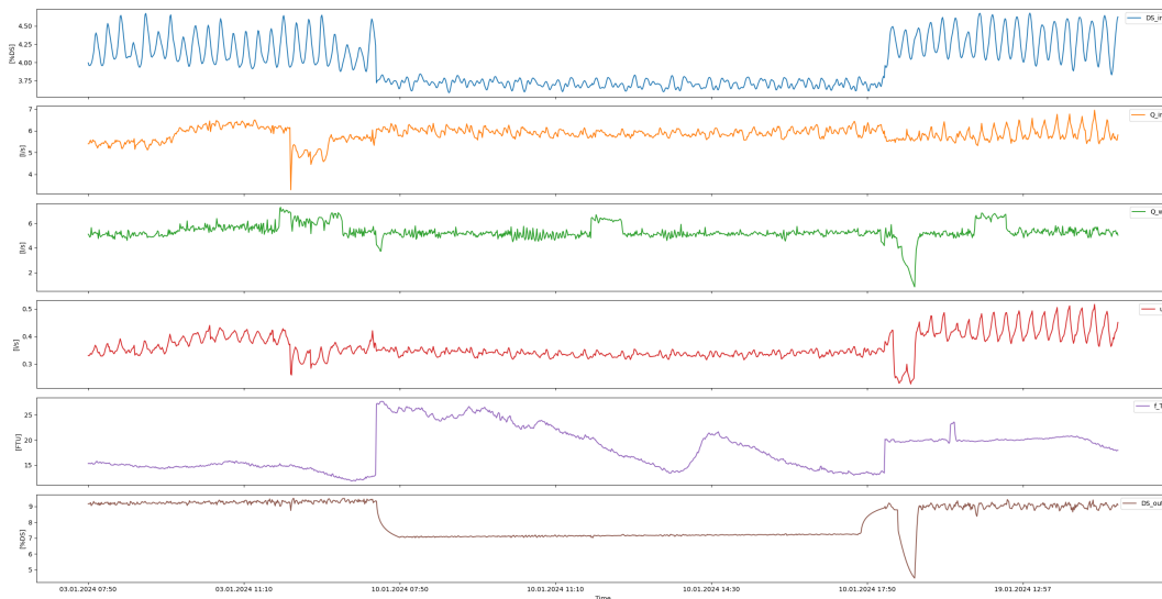
Figure 5.4: Interpolation of dry solids with input variables over 2 days
