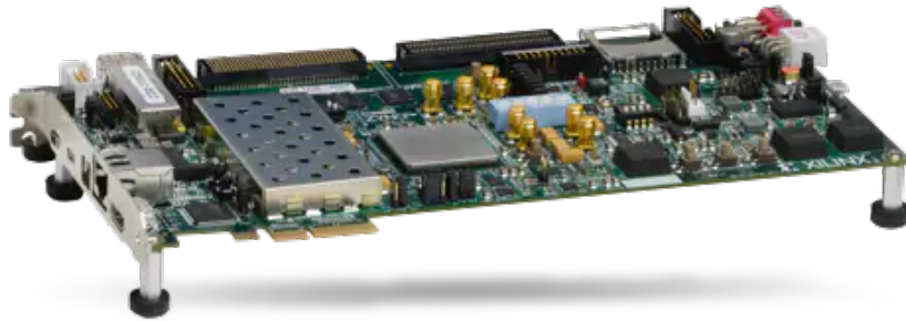
FIGURE 3.3: AMD Zynq 7000 SoC ZC706 Evaluation Kit [91].
