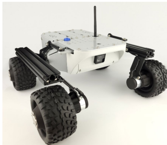
Figure 3-1: A 4-wheel drive-controlled Leo Rover without modifications [11].
