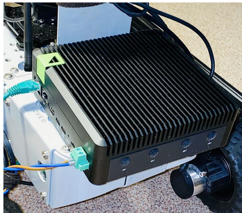
Figure 4-4: Addition computer connected with ethernet cable to the rover.
