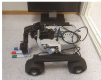
Figure 1: Our Leo Rover robot trying to pick up green objects.
