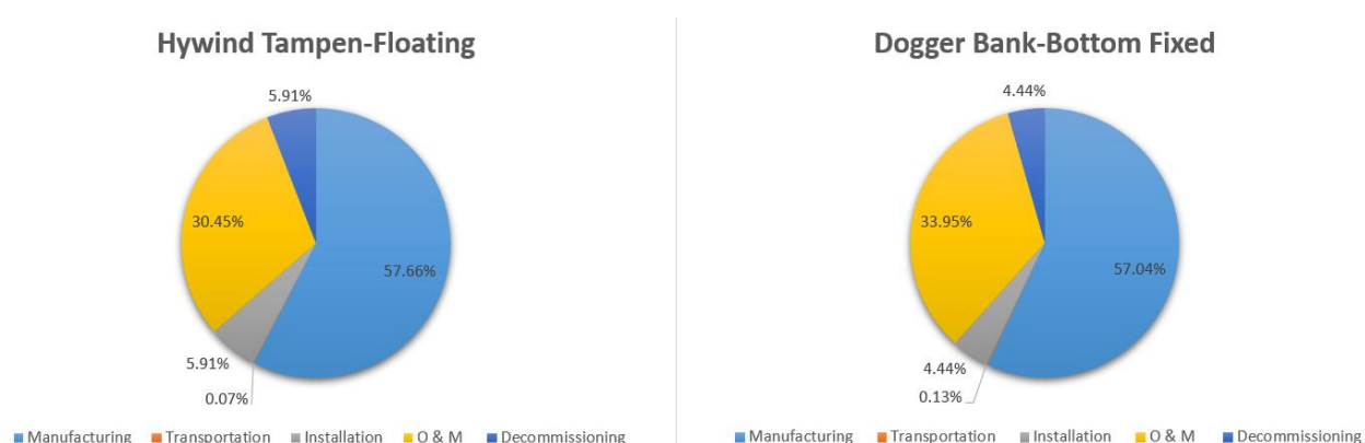
Figure 7.4 Contribution of the main five life cycle stages to total GWP for base case scenarios.
