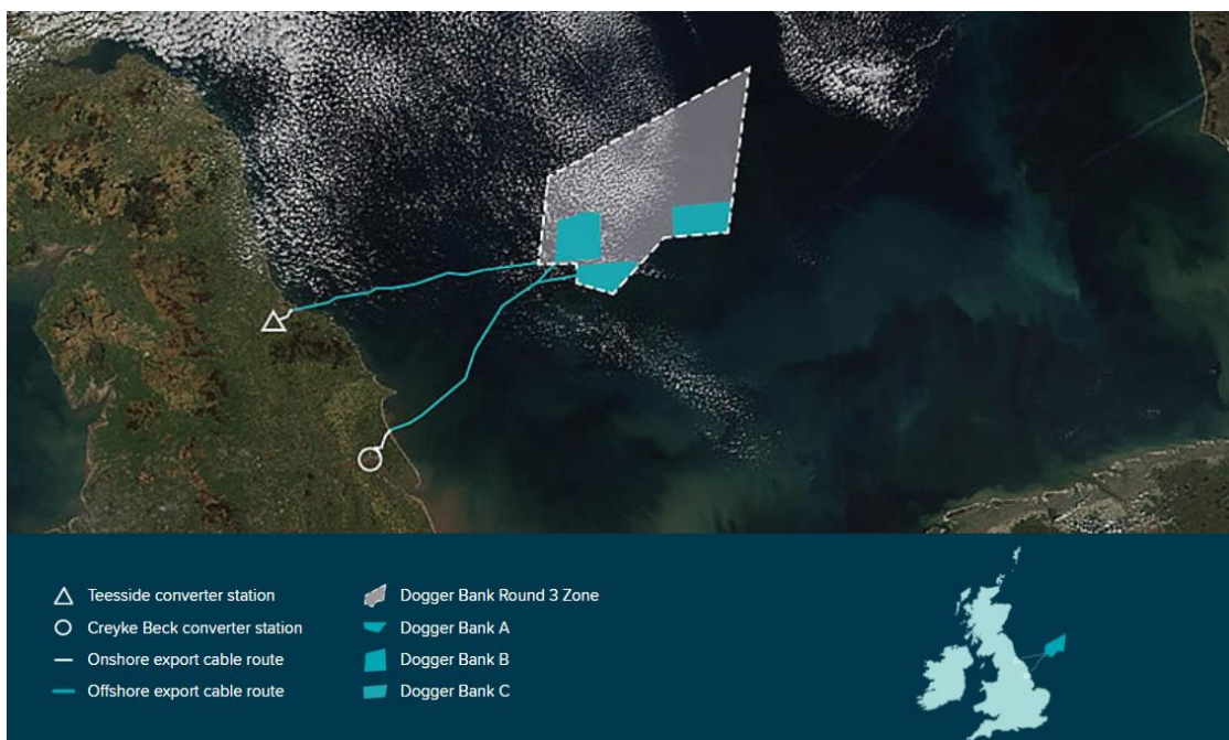
Figure 6.1 The Dogger Bank wind farm layout [67].
