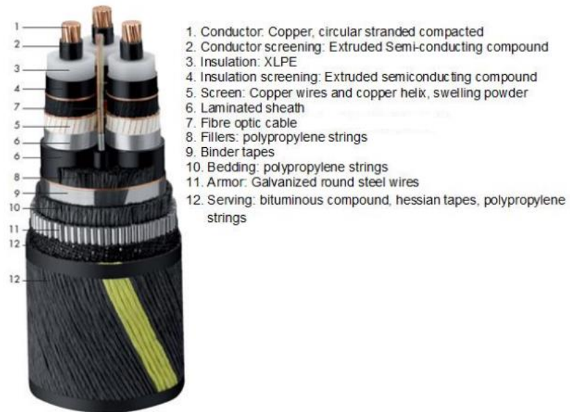
Figure 3.21 Components of a three core cable [54].
