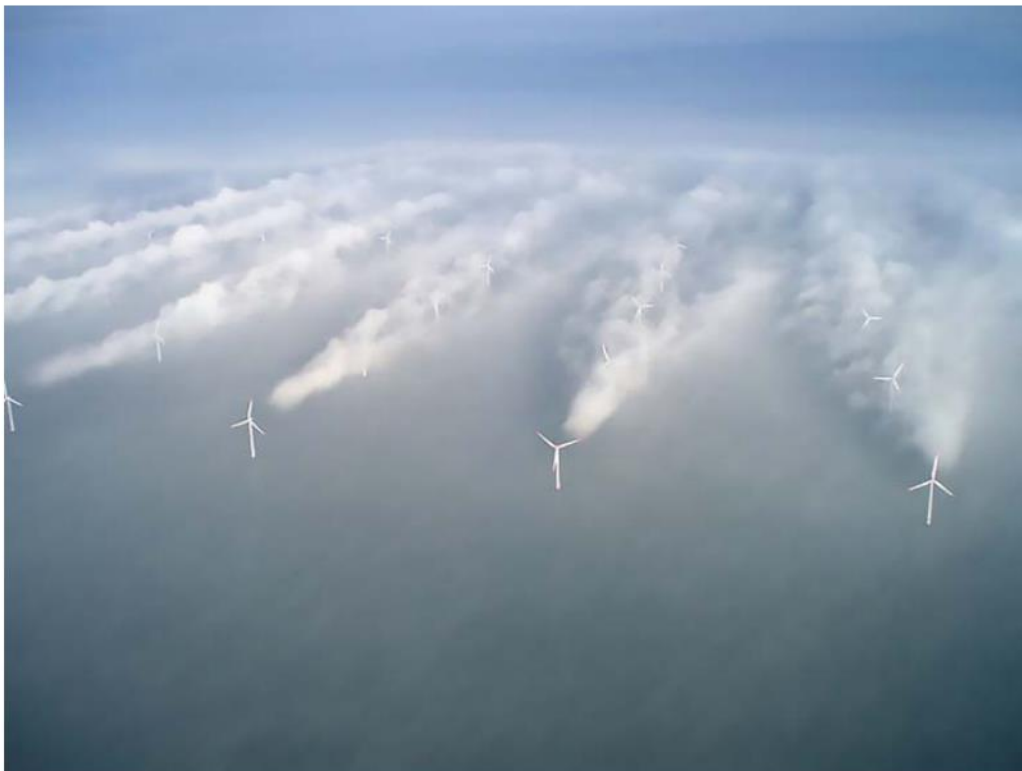
Figure 3.16 Wake turbulence in an offshore wind farm [45].
