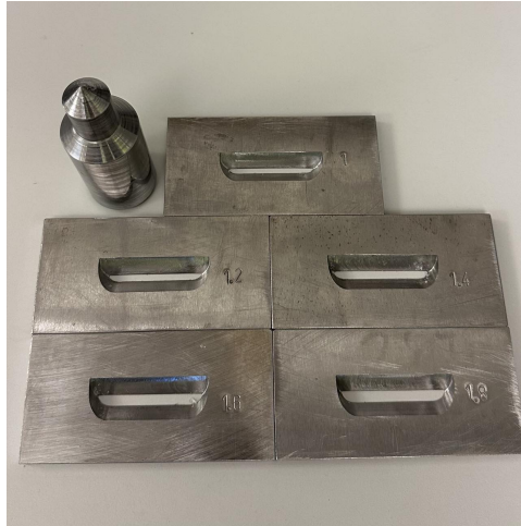
Figure 3.5: The manufactured templates with the custom knife for implementing cuts to the XLPE insulation.
