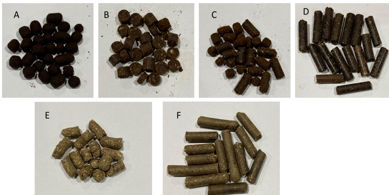
Figure 39: Pellets formed at different operating conditions: (A) only coffee grounds pellets, (B) coffee grounds with coffee grounds (94 wt.%), saw dust (3 wt.%), and bark (3 wt.%) at die temperature greater than 60°C, (C) coffee grounds with coffee grounds (94 wt.%), saw dust (3 wt.%), and bark (3 wt.%) at die temperature 30°C-45°C, (D) coffee grounds with coffee grounds (92 wt.%), saw dust (5 wt.%), and bark (3 wt.%) at die temperature 50°C-60°C, (E) straw at die temperature 30°C-45°C, and (F) straw at die temperature 50°C-60°C,
