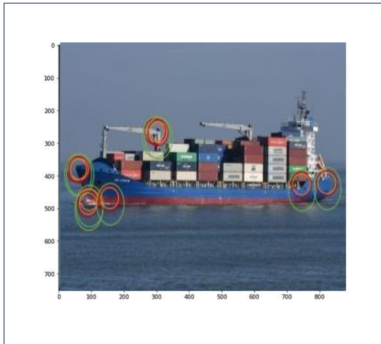
Figure 4. Keypoints detected by the ORB extracted idea from (Rublee et al., 2011)
