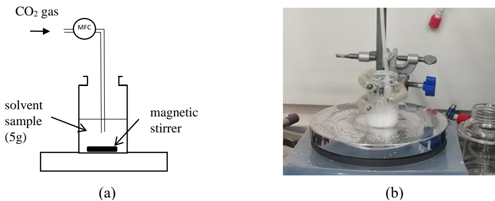
Figure 3: Experimental setup for CO 2 loading and determination of onset of solid formation. (a) Schematic Diagram, (b) Laboratory setup at the onset of solidification.
