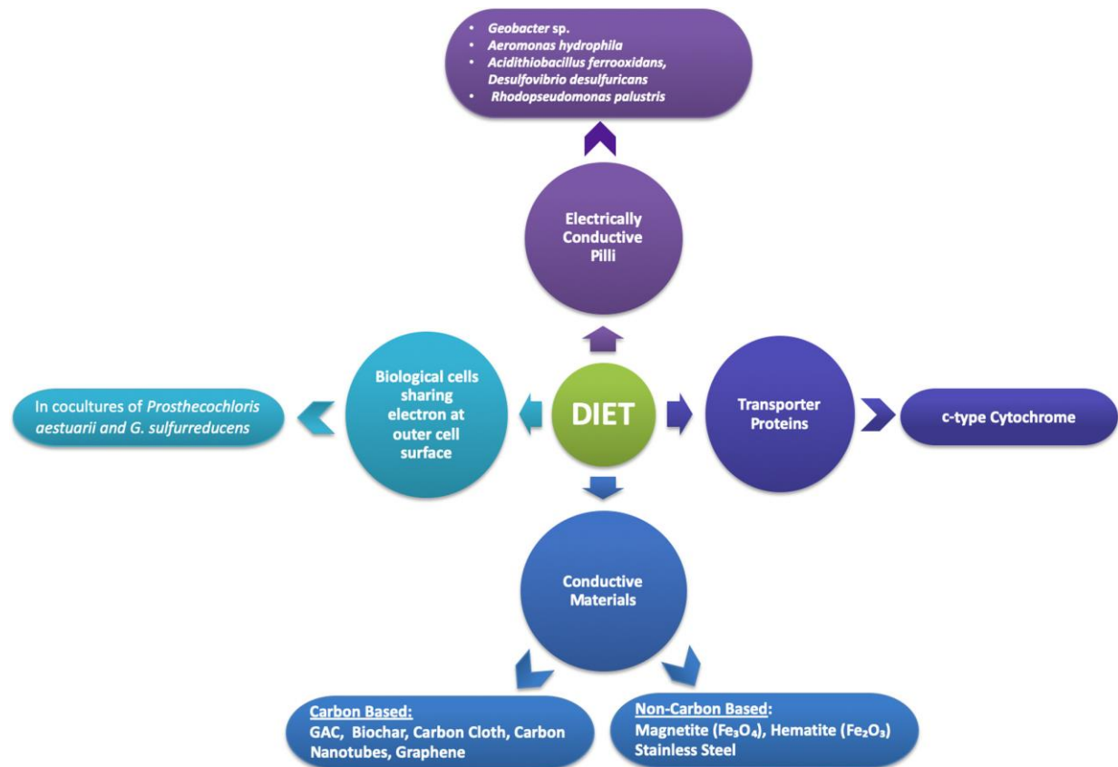
Figure 2.4: Various mechanisms of DIET [32]
