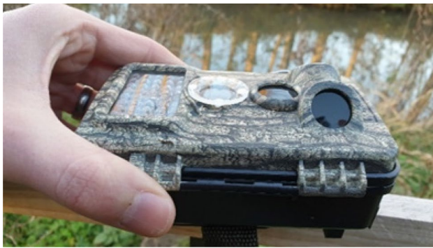
Fig. 3 The external lens of +1 dpt attached to the low-class camera model 2 (L2)
