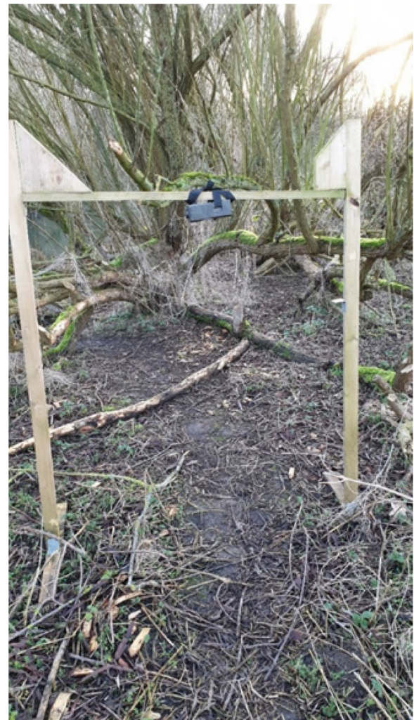
Fig. 2 A camera trap with the recording side pointing downwards fixed to a wooden frame at a recording height of 1.0 m over a beaver pathway
