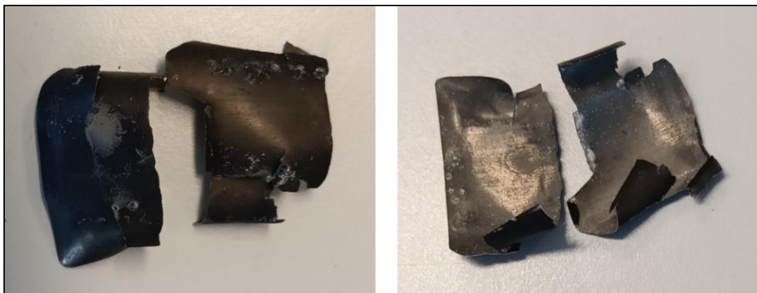
Figure 4.3 Broken electrodes during electrochemical operation.
