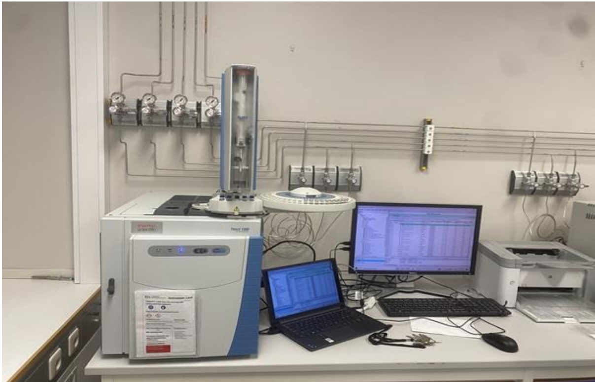
Figure 3.5: Gas chromatograph used for determining the concentration of VFA.
