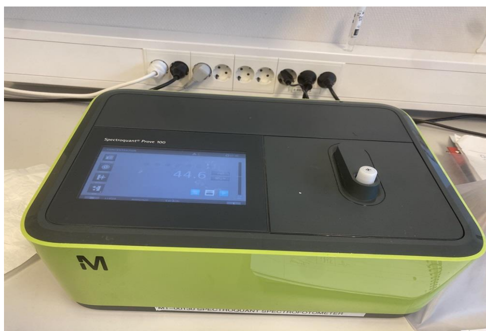
Figure 3.4: Spectrophotometer used for measuring COD and ammonium concentration.
