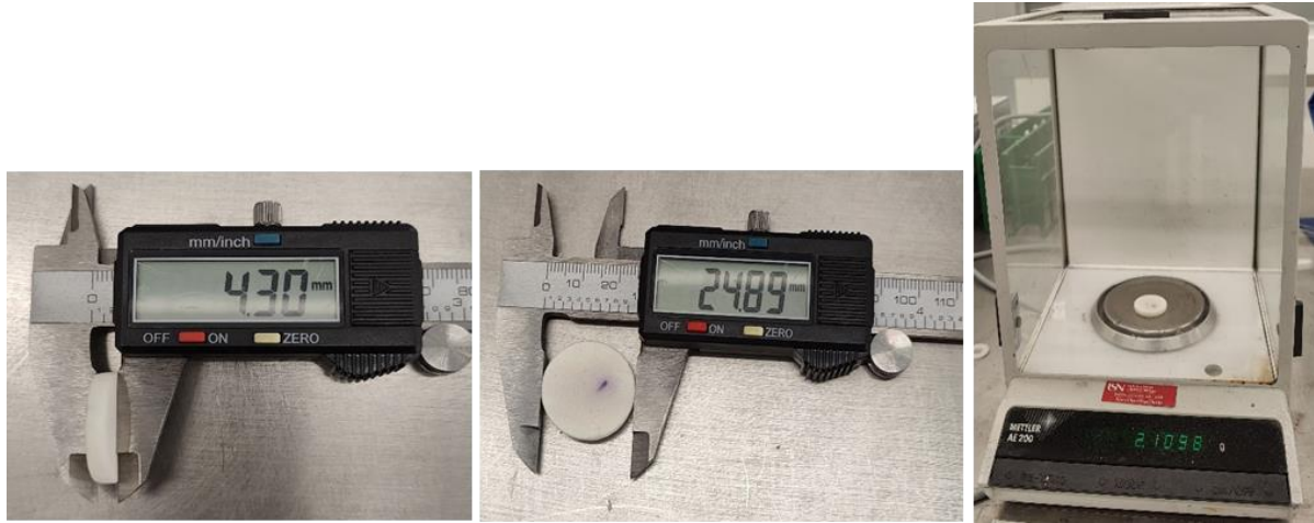
Figure 5 Identification of thickness, radius, and mass using slide calipers and a weighing scale.
