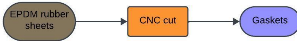
Figure 4. 3: Flow of Gasket Processing
