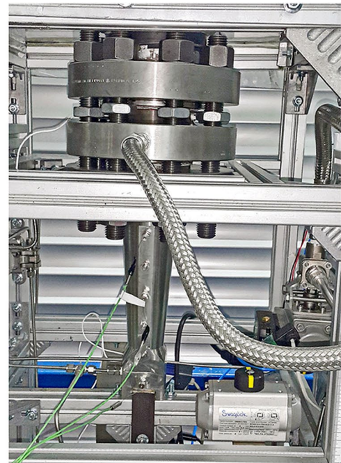
Fig. 1 Schematic drawing of the double-diaphragm conical arrangement, its main dimensions, and a magnified MPS sketch on the left-hand side. An image of the conical vessel fastened with the two flanges on the right-hand side
