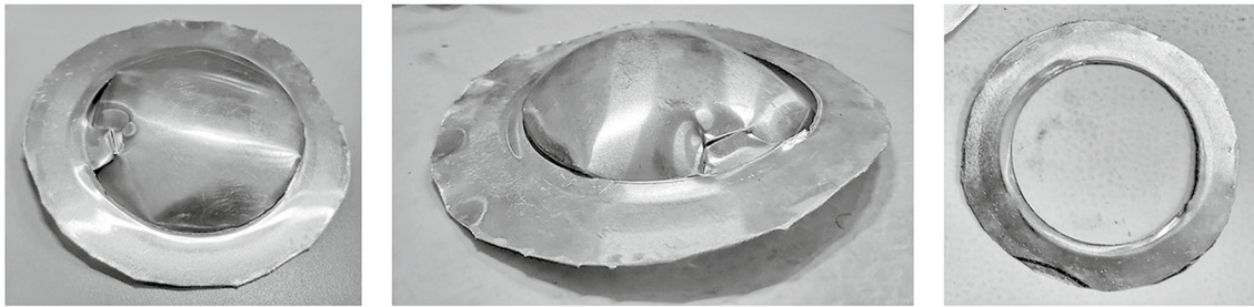
Fig. 8 The left and middle images show circular tracks on the bulged diaphragm circumference after the HP diaphragms were ruptured by MPS pressure relief. The right image shows the remain-
