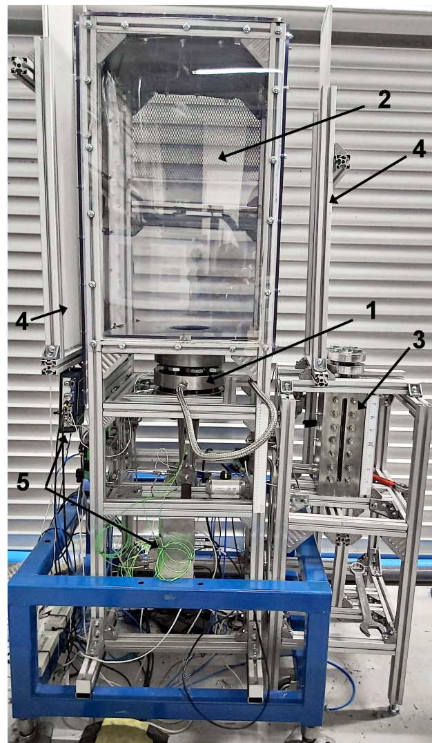
7 Figure 3.1: Double-diaphragm conical arrangement for the accidental release of liquid CO 2 from transport and storage.
