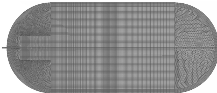
Fig. 2 – Computational mesh for the 2D CFD analysis (Case 1: 2D CFD simulation of small H2-tank).
