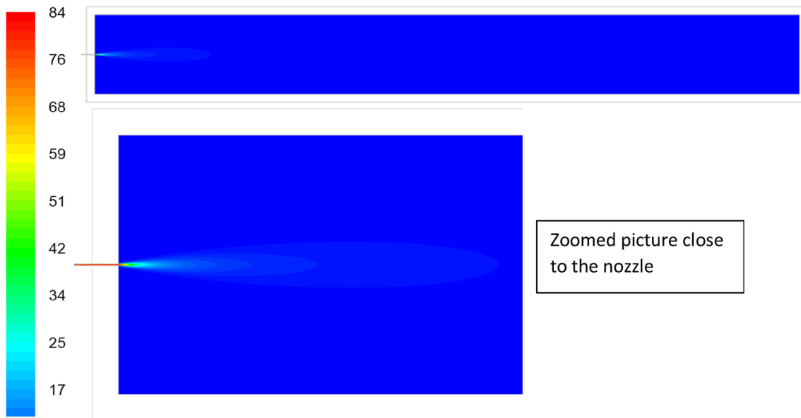
Fig. 14 – Result from 2D CFD simulation of a large H 2 tank. Velocity magnitude distribution inside the tank at 20 min time instance. Velocity values are shown in m/s.
