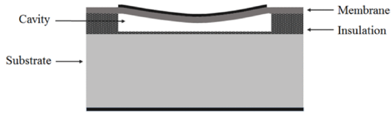
Figure 2 - 4 Basic CMUT Cell [31].
