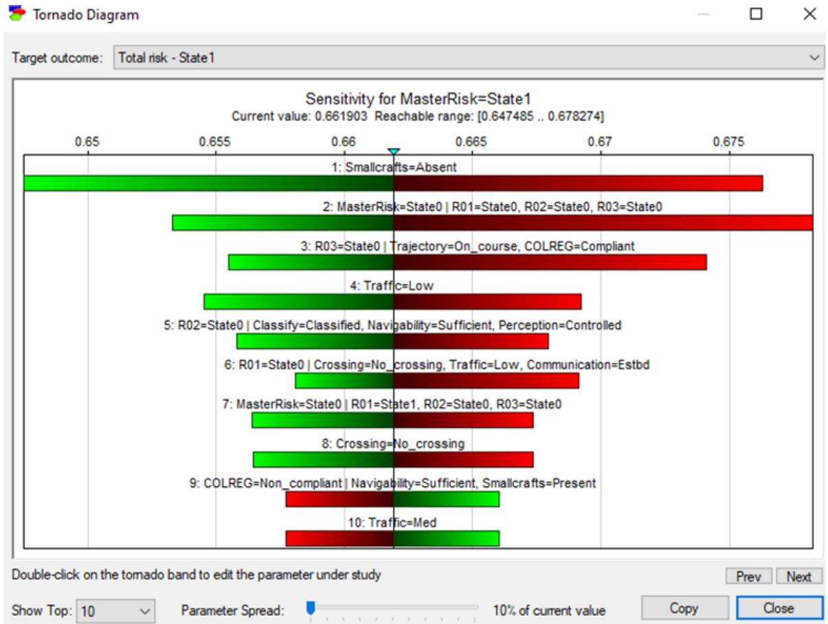
Figure 37 - Sensitivity analysis - BN model: Tornado diagram (with node variable names)
