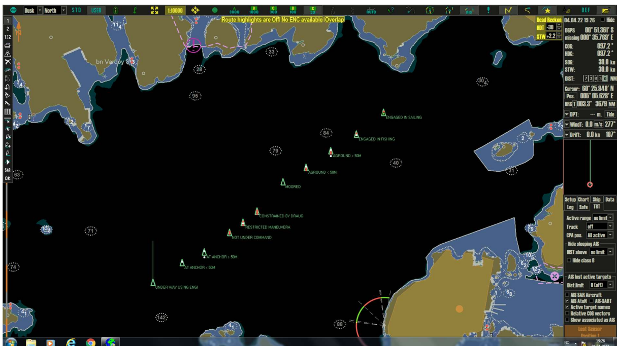
Figure 8-2: Descriptive picture before the start of the SAGAT tasks. ECDIS in dusk mode. AIS symbols with lanterns.
