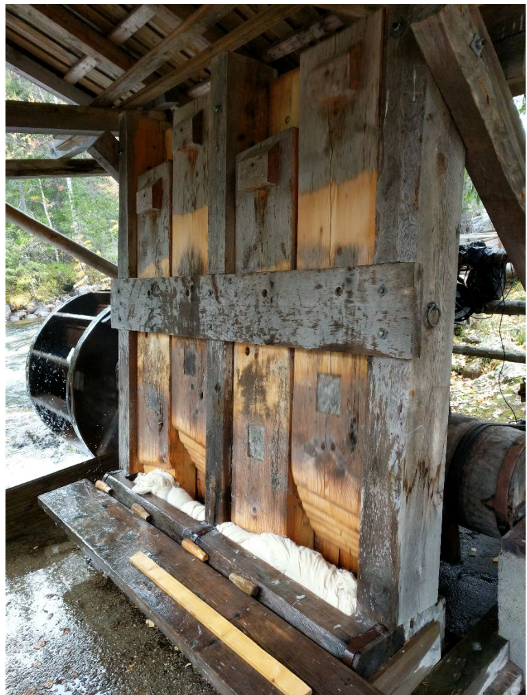
Image 1 The fulling mill at Mjonøy, with the weaving class's wadmål being fulled
