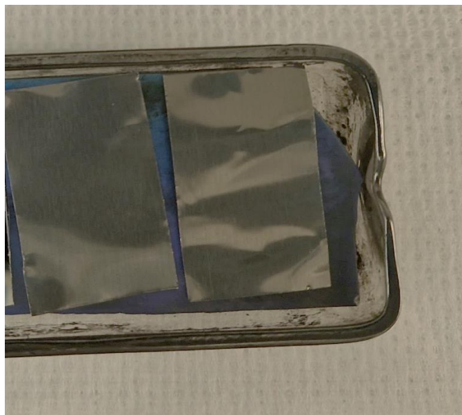
Figure 3-2: 70 \mu m Al substrate with a sputtered Ni layer of 100nm machine specified planar surface thickness.
