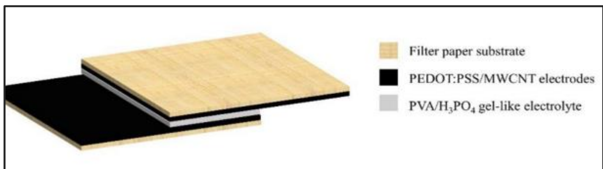
Figure 2.6: Supercapacitor schematic illustration to show the assembly and architecture of SC [33]
