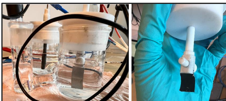
Figure 3.6: Visualization of 3 electrode setup based on Counter Electrode, Working Electrode Reference Electrode
