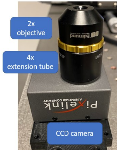
Figure 4-6 Objective lens, extension tube, and CMOS camera
