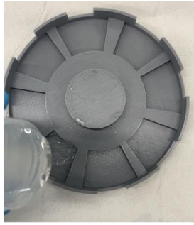
1. Pour well-mixed PDMS onto the holder bowl up to 4mm height
