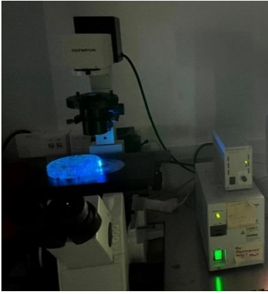
Figure 2-7. MVX10 microscope with a blue excitation source and detection from the side view. The illumination source is positioned above the sample stage glass, with the sample exposed to vertically illuminated excitation light. The detector is located at a side view angle corresponding to the fluorescence illuminator, to capture and analyze the emission light emitted from the sample.
