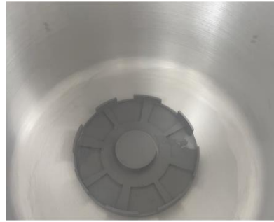
2. Vacuum the substrate molding at -0.8 Bar in 20 minutes
