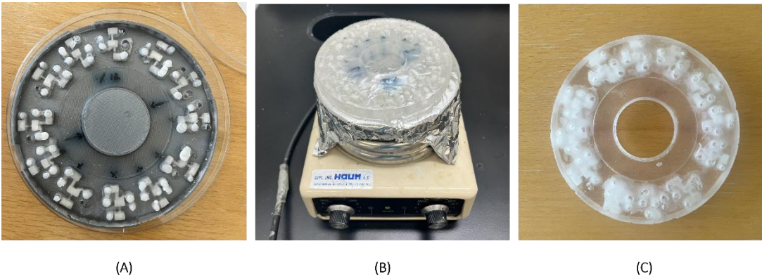
Appendix. 4 (A) The cured paraffin inside the structure. (B) The paraffin is melted on a hot plate. (C) The device after injecting the melted paraffin.
