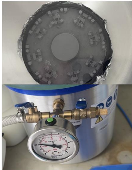
4. Vacuum the whole structure at -0.8 Bar in 20 minutes
