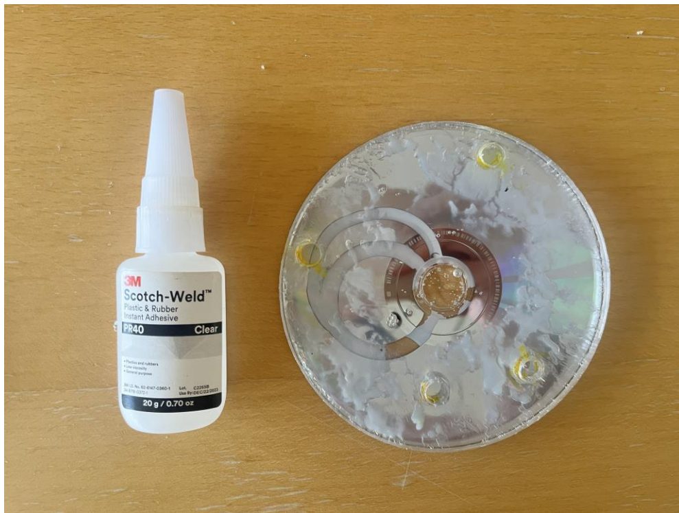
Appendix. 1 The 3M adhesive glue and its white pattern resulted on the device.
