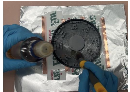
2. Apply a cooking oil layer on the structure mold
