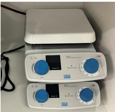
Figure 2-8. The AREC hot plate. This version has both heating and magnetic stirring functions. Only the heating function is used in this project.
