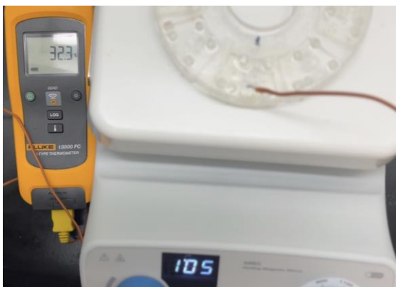
Figure 4-5. Incubation on the hot plate. The lab-on-a-disc is loaded on the hotplate with a set temperature of 100°C. The temperature on the surface of the processing chip is measured with FLUKE t3000FC K-TYPE THERMOMETER, which is 32.3°C.
