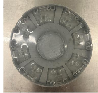
3. Slightly press the PDMS sheet on the substrate mold and cure at RT, 48 hours
