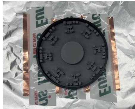
1. Glue the structure mold to the Al foil with double-sided tape
