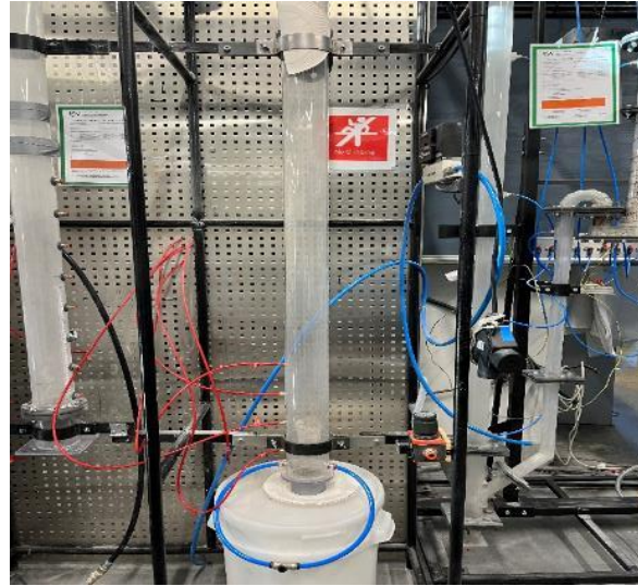
Figure 4.5 Fluidized bed reactor with two side nozzles as inlet boundary conditions.
