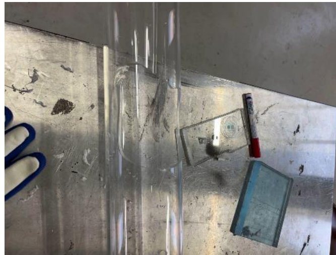
Figure 4.4 Breakage of the tube during drilling by normal bit.
