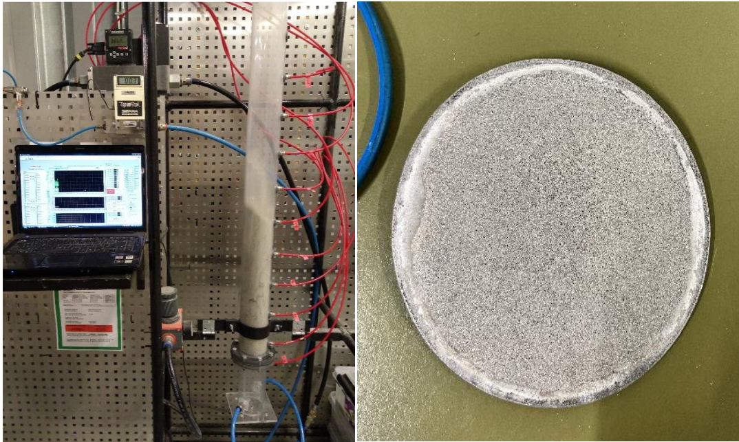
Figure 4.5: (a) Left fluidized bed reactor with distributor plate, (b) Right distributor plate.
