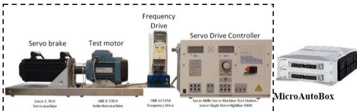
Figure 3.1: The servo test stand, where the striped box shows the servo test stand provided from Lucas-Nulle.
