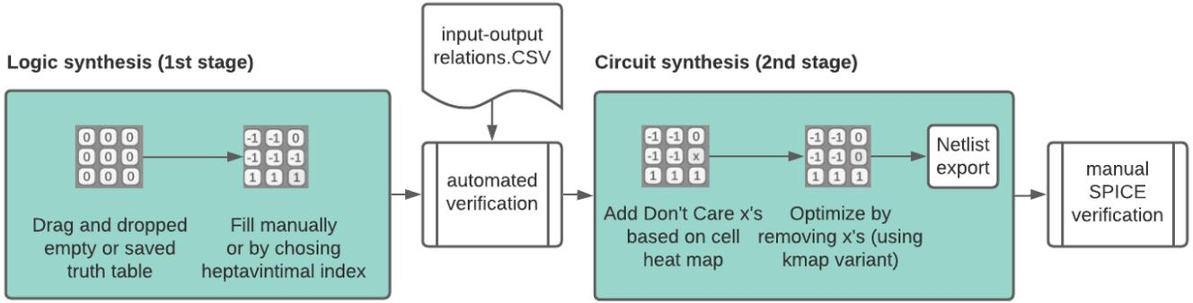
Fig. 3: **Design flow.** Two stage design with simulation and verification
