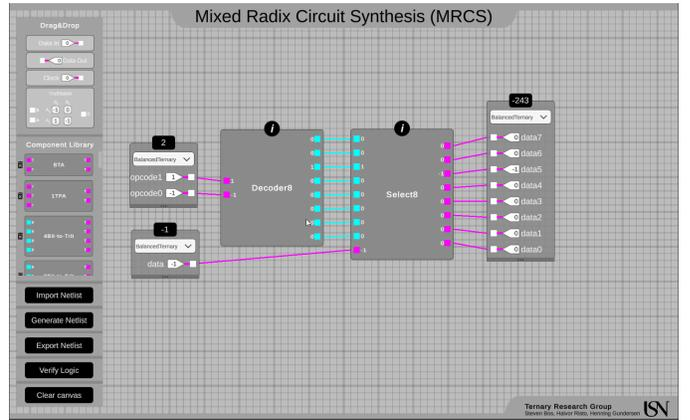
Fig. 2: **Main user interface.** The decoder8 and select8 components are part of a 8:1 balanced ternary multiplexer component that is shown at abstraction level 1. Circuits can be stored as components in the component library and become part of larger logic networks/hierarchies. Fig. 4 shows a binary SR latch component at abstraction level 0, the lowest.
