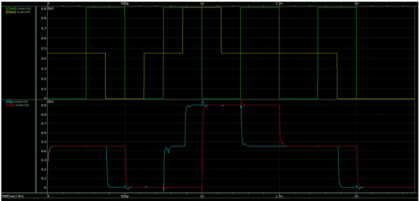
Fig. 7: HSPICE Transient analysis without load. (Top) Binary clock and ternary data signals. Clock frequency is 2 GHz. (Bottom) Flip and Flop signals. Note that in high clock periods the Flip latch copies the data signal, while in low clock periods the Flip latch is disconnected and the Flop latch copies from the Flip latch.
