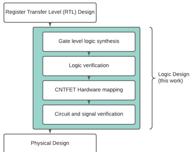
Fig. 1: **Scope of this work.** Logic design of CNTFET-based binary, ternary and mixed radix integrated circuits
