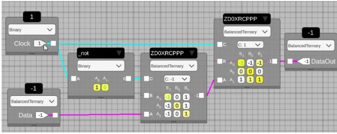
Fig. 5: **Balanced ternary flip-flop.** Rising edge (RE) master-slave (MS) configuration. A single D latch is 18 transistors and requires 5 inverters of 2 transistors that can be shared with multiple components for a total of 28 transistors. The flip-flop uses a total of 54 transistors since 1 inverter is shared between two inputs. An equivalent 8 NAND + 2 inverter binary flip-flop design uses 36 transistors.
