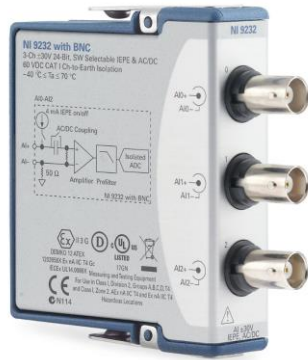
Figure 14: NI 9232 with three channels is used for data acquisition of the accelerometers
