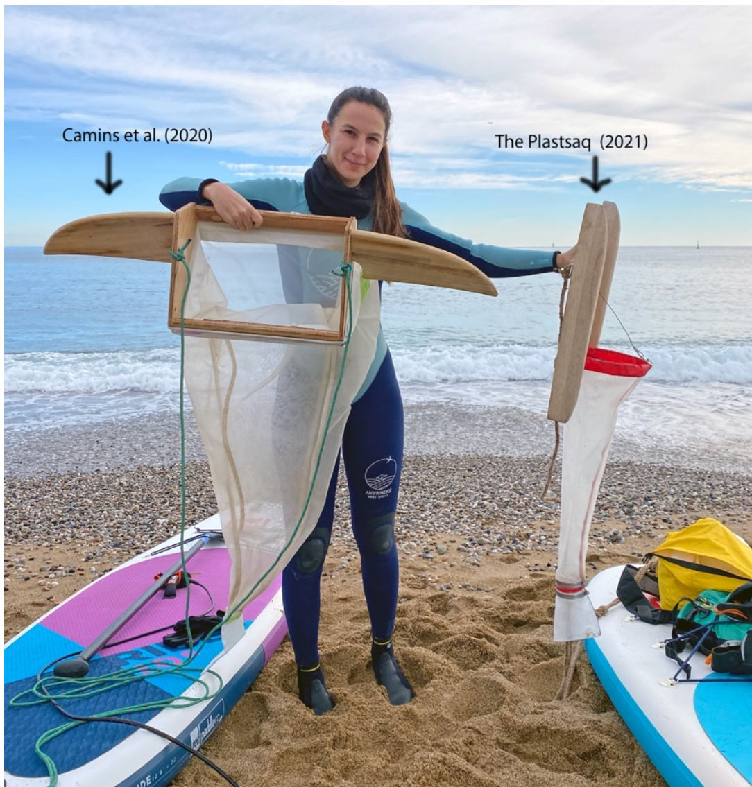
Figure 3 - Laura Galeano (Bachelor student UiB) holding the Camins et al., (2020) sample device and our trawl “the Plastsaq” at Barceloneta Beach (Spain). In this nearshore area close to Barceloneta beach in Barcelona we sampled the two-trawls side by side on a simultaneous sample. Photo: Kristian Louis Jensen
