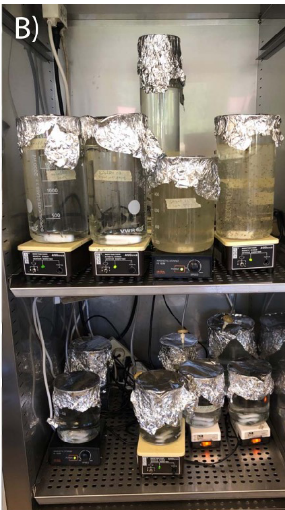
KOH: NaClO added to sample liquid in heating cabinet under constant agitation
