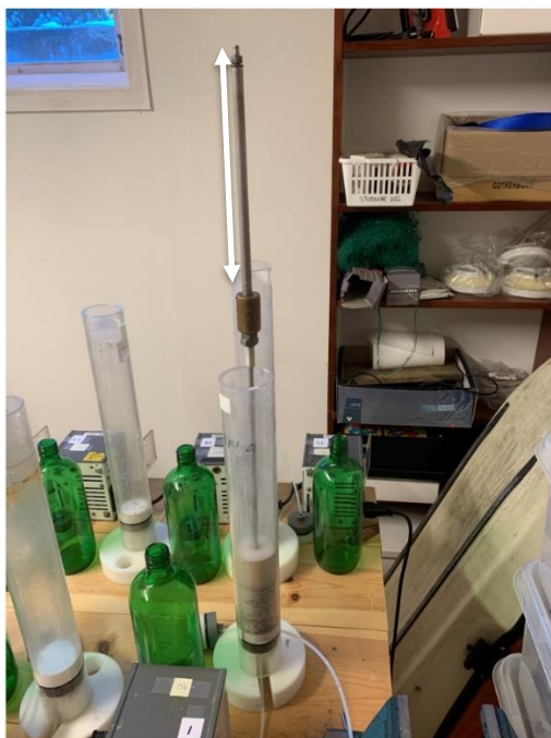
Figure 4: Packing of the 2.5 cm layers in the column using a rammer of 125 g. White arrow shows up/down movement of the rammer.
