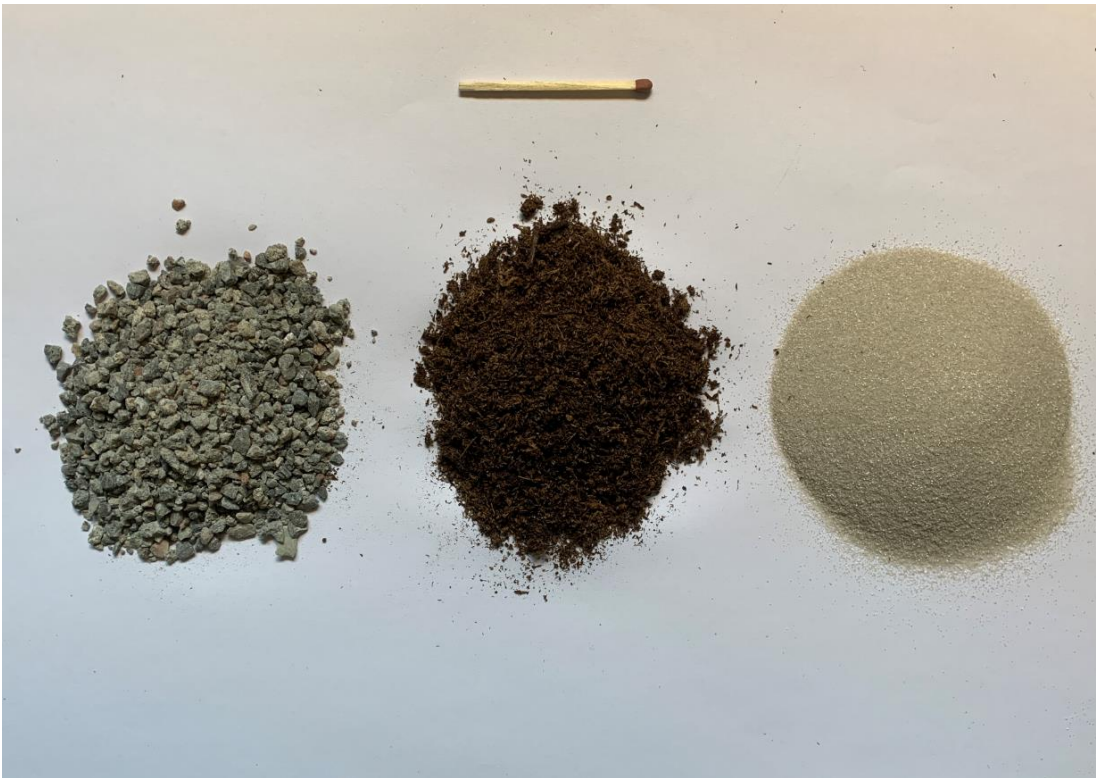
Figure 1: The prepared materials used in in the leakage experiments. From the left; concrete (RCA), soil (peat) and sand.
