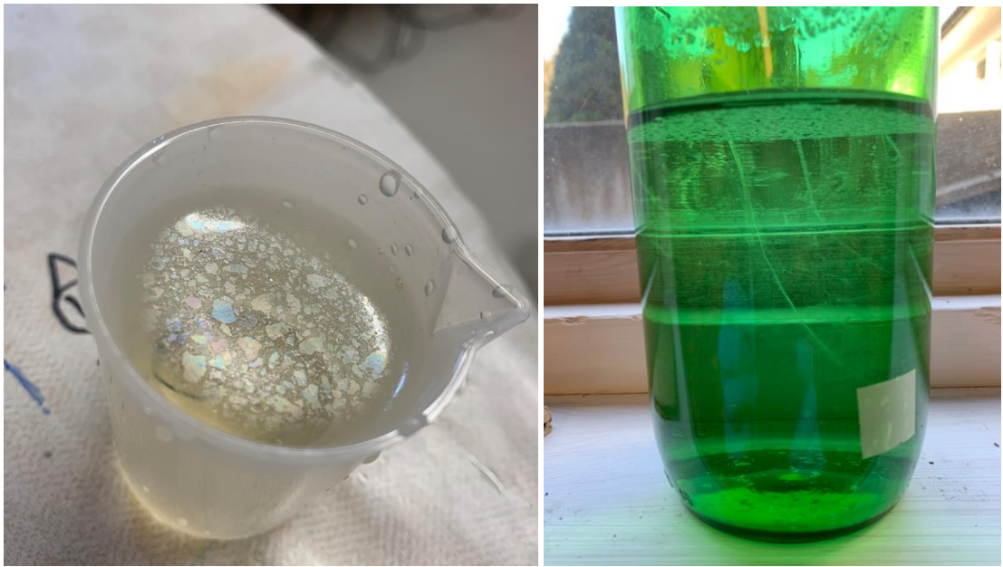
Figure 14: A film (right) was observed on top of the water eluate bottles (except for the blanks “Sand” and “Soil”) which formed flakes before precipitating to the bottom of the bottles. A coating was also formed inside the bottle walls. A film (left) was formed spontaneously when the water eluate was transferred to a beaker.
