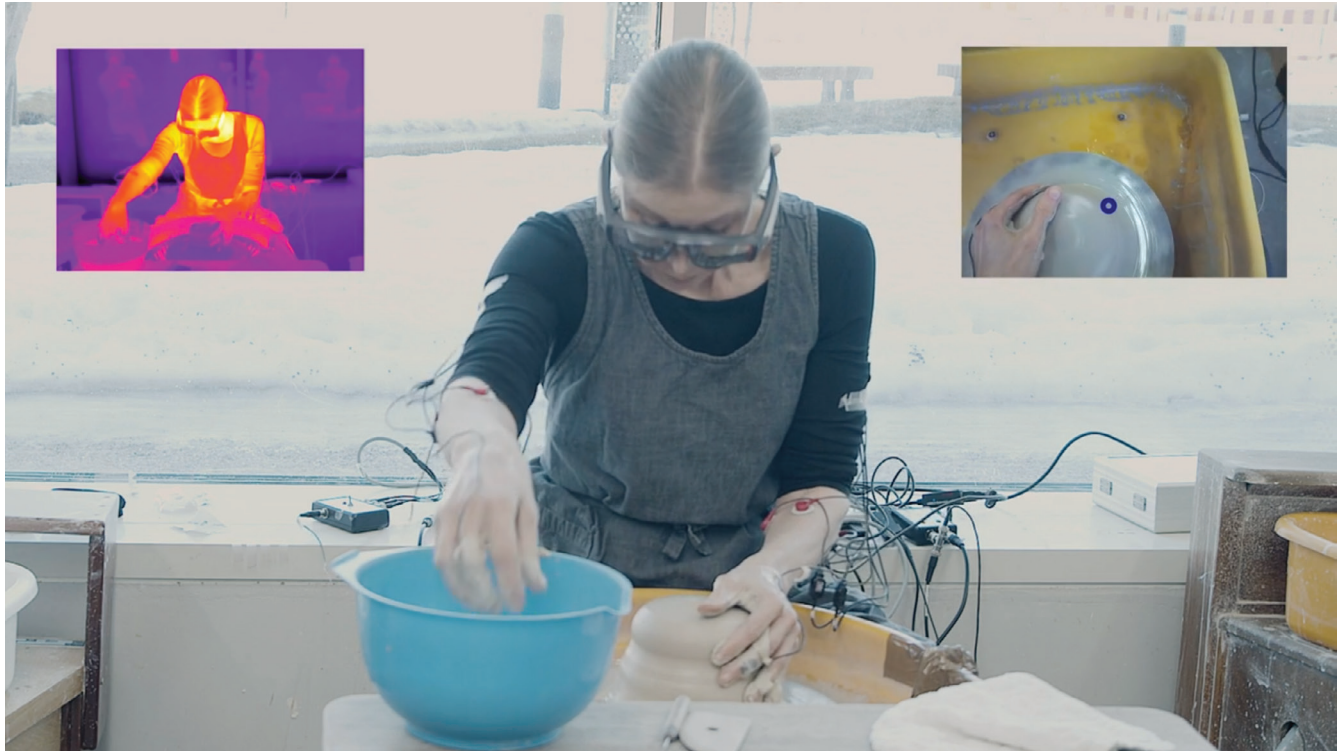
Figure 1: The setting of the current study. The craft researcher–practitioner wears action monitoring equipment while throwing clay. This screenshot is from the actual video, and the inserts show simultaneous views of the thermal camera (upper left corner) and eye-tracking scene camera (upper right corner). Electromyography electrodes and wires are visible on both forearms, and accelerometers are seen on the fingers. In addition, the rotation velocity of the throwing wheel was monitored simultaneously (not shown in the figure). The images are from a video was taken by Iikkamatti Hauru at the Aalto Studios: https://studios.aalto.fi/ . Accessed 26 July 2022.
