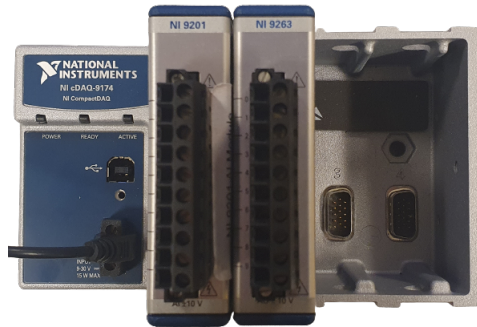
Figure 4.4: National Instruments compact Data Acquisition
