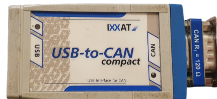
(b) IXXAT USB to CAN adapter
