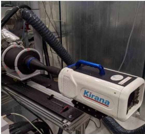
Figure 3.3. KIRANA ultra-high-speed video camera with telecentric lens
