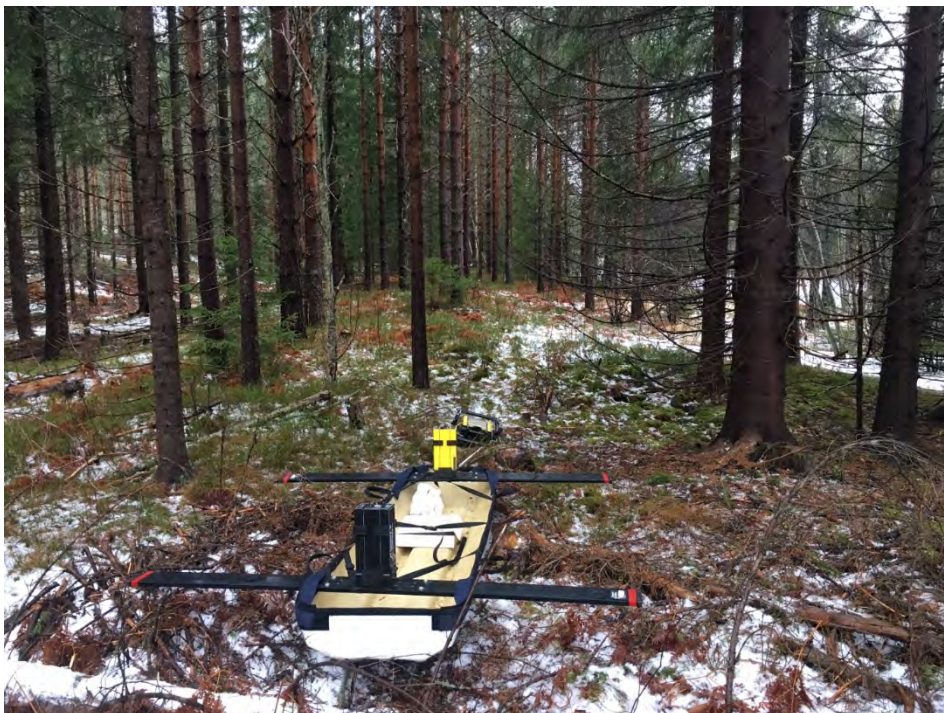
Figure 3-2. GPR fieldwork with 50MHz antennas on profile 5.
