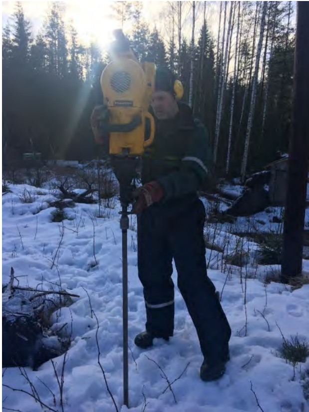
Figure 3-3. Probe drilling performed at profile 6 by Frode Bergan
