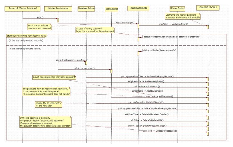
Figure 3: SD for Maintain Configuratin from Node-RED UI.
