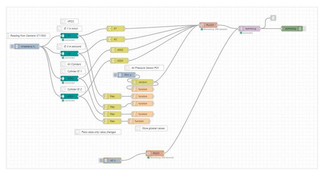
Figure 1: Node-RED flow for Test Celle machine and simulated Packaging Machine 03 (PM03).
