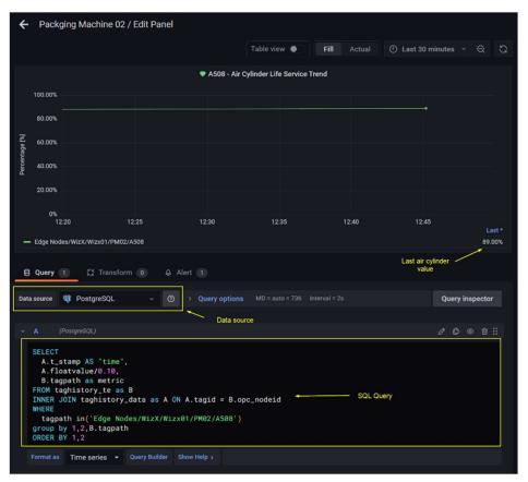
Figure 5: Graph panel for A508 air cylinder shows the query tab window that fetchs real-time data from data source.
