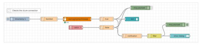
*Figure 4: Flow that checks the connection with the database server in Azure.*
