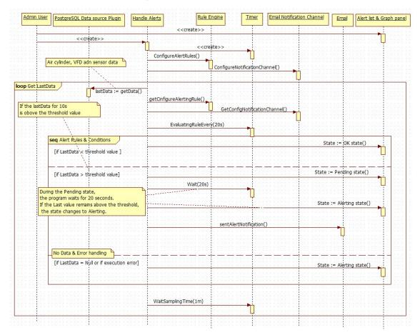
Figure 2: Handle Alerts Sequence Diagram (SD).
