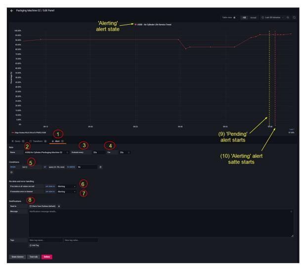
*Figure 6: Alert configuration window for A508 air cylinder.*
