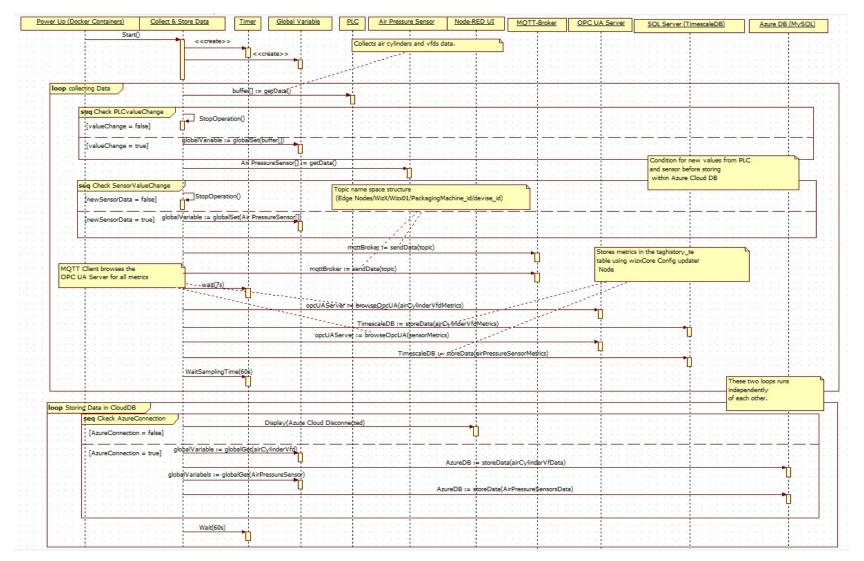
Figure 1: SD for Collect and Store data use case.
