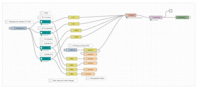
Figure 2: Node-RED flow for collecting data from the PLC, air pressure sensor simulator and sends to MQTT Broker and at the same time stored a global variables.
