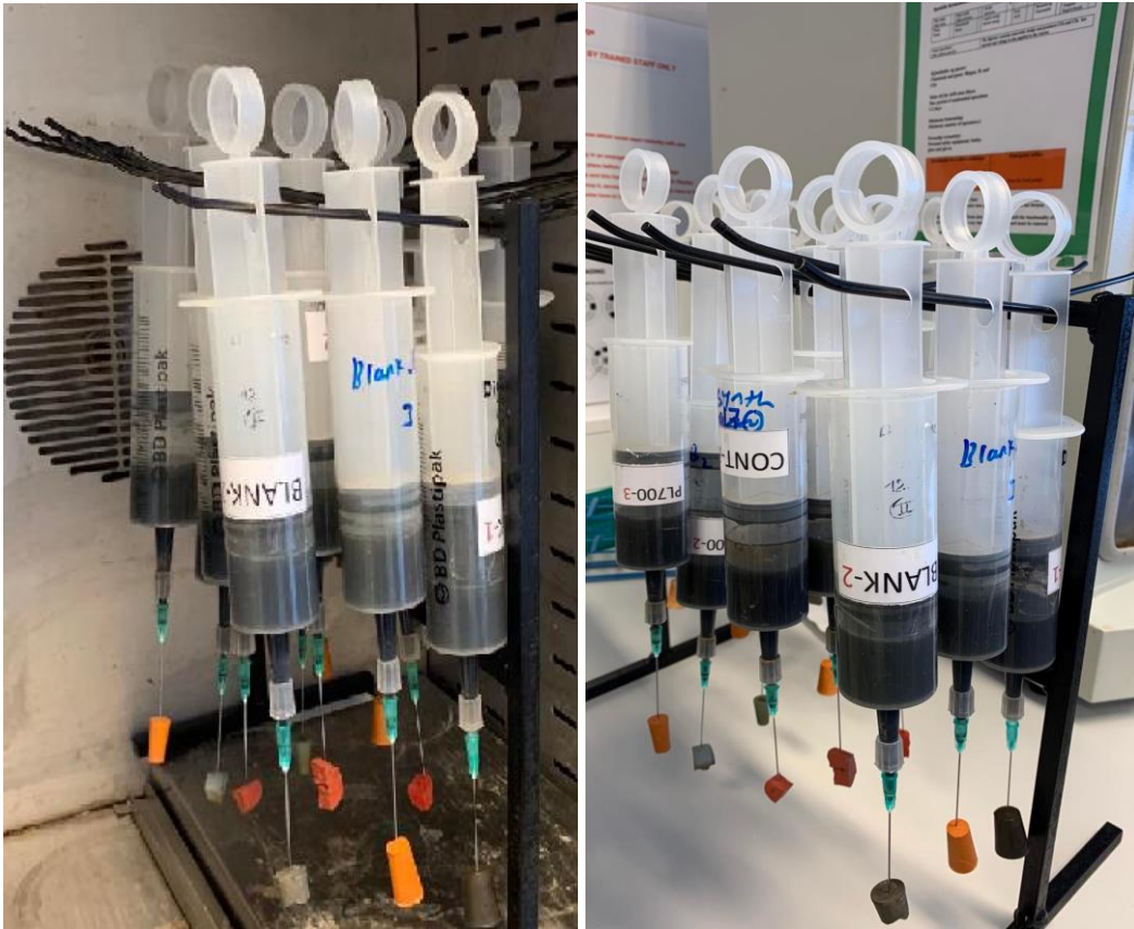
Figure 3.4: BMP syringe test with inoculum and substrate (apple juice & APL)
